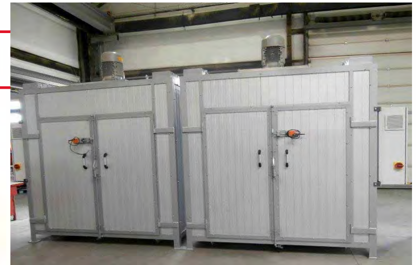
Chamber drying furnaces
