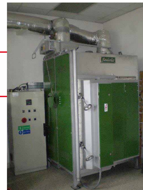
Chamber kilns for glass cooling
