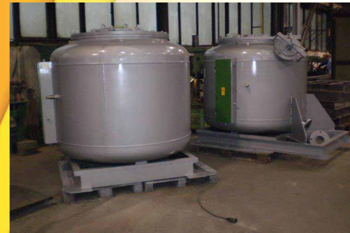
Holding furnaces for low pressure casting
