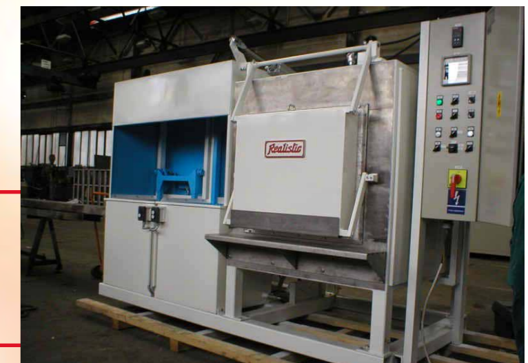
Chamber furnaces and quenching tanks
