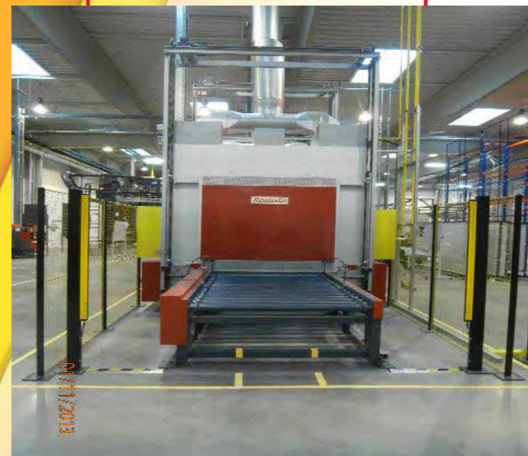
Continuous furnaces with roller conveyor
